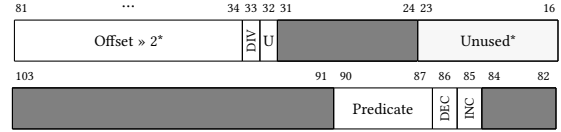
Figure 10: BRA instruction on 80 \leq SM < 90 (Ampere). For SM \geq 90 (from Hopper), the first 8 Unused* bits encode the LSB of offset \gg 2 and bits 34-81 encode offset \gg 10
